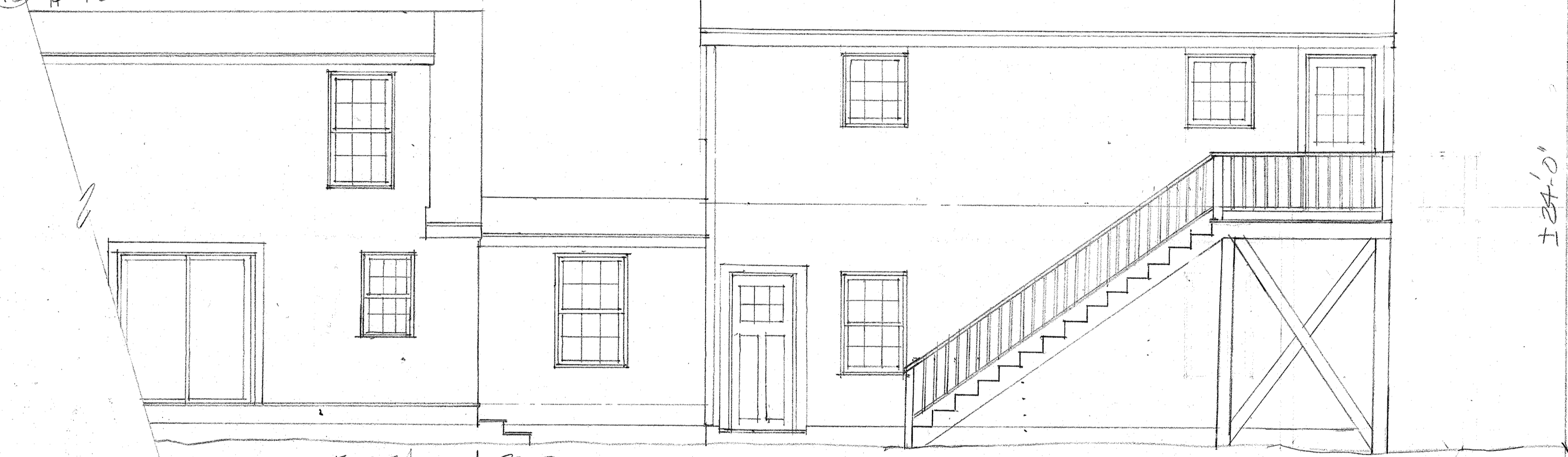
2 EAST ELEVATION @ GARAGE & MIDROOM A2 1/4" = 1'-0"
